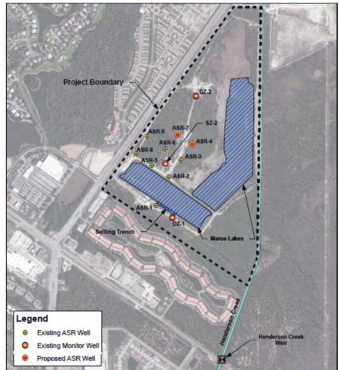
At right: Figure 2. Aquifer Storage and Recovery Wellfield at the Source Water Facility
